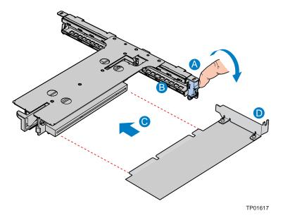
Figure 35. Installing an Add-in Card to the PCI Riser Assembly
